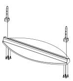
Assemble the PDP with the stand and firmly secure the PDP using 4 screws provided.
