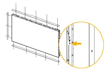
Before mounting the set's outer cover after installing a Video Wall or Samsung UD, remove the stickers attached to the connecting screw holes first.
